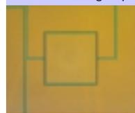
The pixels easily meet the noise equivalent power (NEP), speed, and power handling requirements for SCUBA-2. Dark NEPs of  $\sim 3 \times 10^{-17}$  W/√Hz have been measured for devices with transition temperatures of 130mK.
