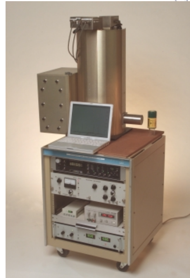
2 stage ADR 6-8 hours operation below T_c
