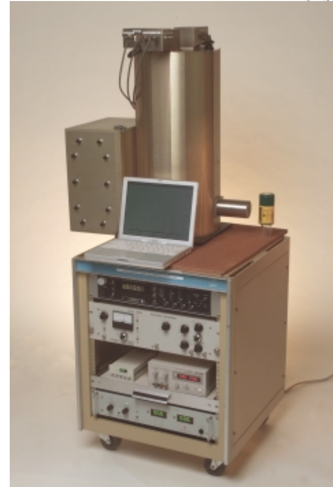
2 stage ADR 6-8 hours operation below T_c
